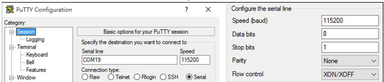
Figure 32 Baud Rate Setting of Serial Connection
