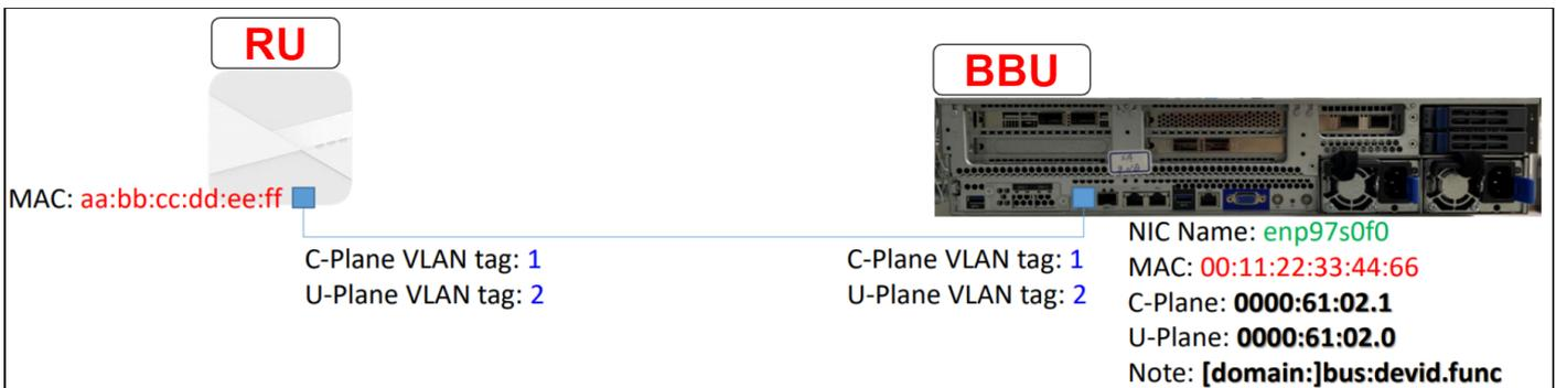
Figure 21 Set BBU MAC Address to Be Connected with RPQN O-RU
