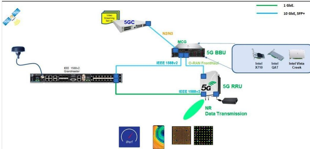
Figure 8 SA L5G System Architecture
