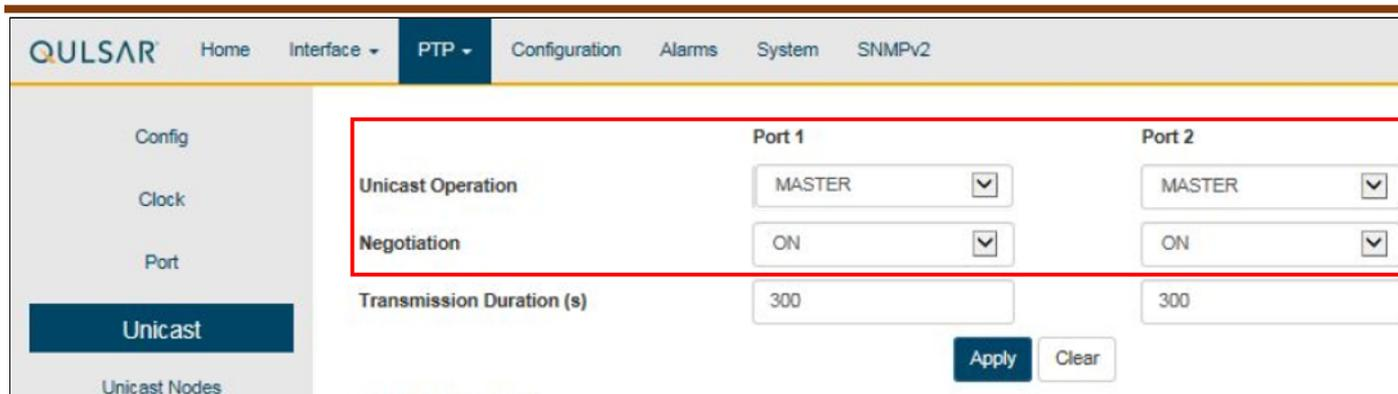
Figure 17 PTP Clock Source Set to Unicast Operation
