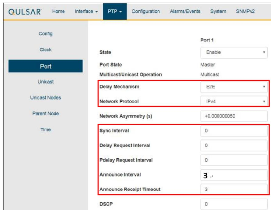
Figure 16 PTP Clock Source Port Setting
