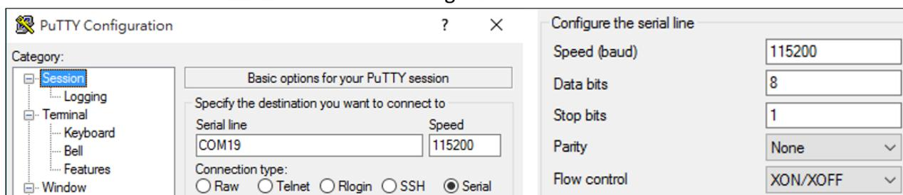
Figure 19 Baud Rate Setting of Serial Connection
