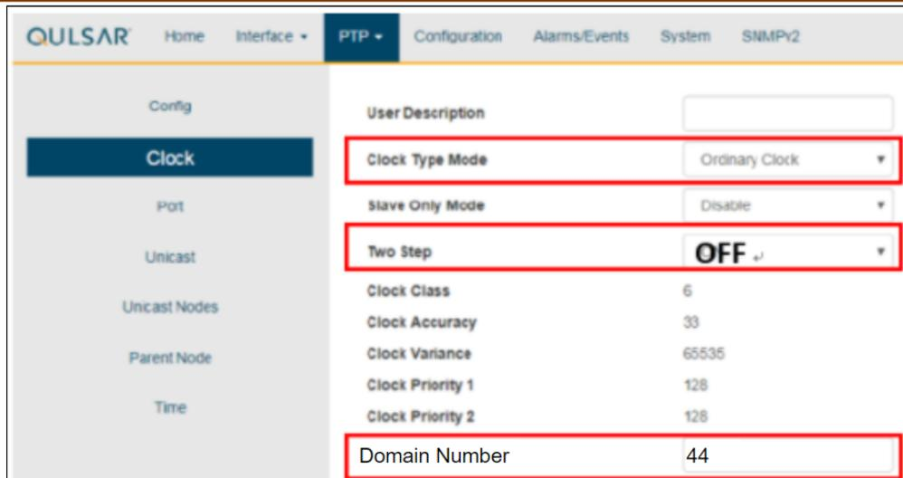
Figure 15 PTP Clock Source Parameter Setting
